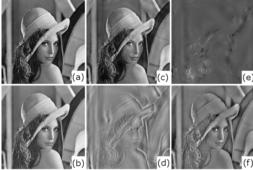
Figure 3: The object wave field reconstruction, L = 10 , z_1 = 1.5 \cdot z_f : (a) |\hat{u}_0| , AM , RMSE = 0.01 , (b) \hat{\phi}_0 , PM , RMSE = 0.1 , (c) |\hat{u}_0| , AM , RMSE = 0.04 , (d) \hat{\phi}_0 , AM , RMSE = 0.192 , (e) |\hat{u}_0| , PM , RMSE = 0.14 , (f) \hat{\phi}_0 , PM , RMSE = 0.172 .
