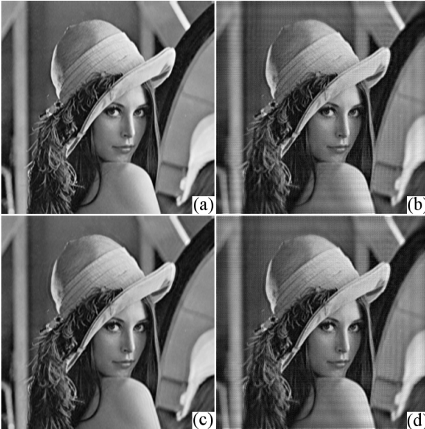
Figure 3.6: Amplitude reconstruction (AM, Lena test-image) obtained using the regularization by truncation, Eq. (3.55), \tau_x = \tau_y , for different distances, noisy and noiseless data: (a) z = z_f , \tau_x=256 , \sigma=0 , RMSE= 1.6 \cdot 10^{-14} ; (b) z = z_f , \tau_x=219 , \sigma=0.01 , RMSE=0.0344; (c) z = 1.15 \cdot z_f , \tau_x=233 , \sigma=0 , RMSE=0.0118; (d) z = 1.15 \cdot z_f , \tau_x=209 , \sigma=0.01 , RMSE=0.039.
