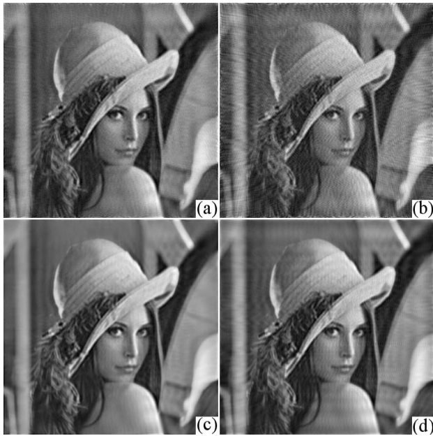
Figure 4.7: Amplitude reconstruction by MF-DDT and AL (100 iterations) from noisy and noiseless measurement data for z = 2 \cdot z_f , K = 5 , AM. The first row corresponds to the amplitude estimates reconstructed from noisy data ( \sigma = 0.02 ) by (a) AL P4 , \mu = 0.0025 , \text{RMSE}(|\hat{\mathbf{u}}_0|)=0.048 and (b) MF-DDT P3 , \mu = 0.05 , \text{RMSE}(|\hat{\mathbf{u}}_0|)=0.062 . In the second row there are results obtained from noiseless observations: (c) AL, \mu = 0.0005 , \text{RMSE}(|\hat{\mathbf{u}}_0|)=0.041 and (d) MF-DDT, \mu = 0.025 , \text{RMSE}(|\hat{\mathbf{u}}_0|)=0.044 .
