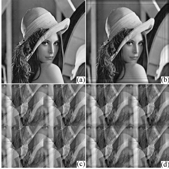
Figure 3.3: Amplitude reconstruction for the close distance z = \frac{1}{2} \cdot z_f , AM, Lena test-image. The results are obtained (a) by the inverse M-DDT as |\widehat{\mathbf{U}}_0| = |\mathbf{A}_x^{-1} \mathbf{A}_x \cdot \mathbf{U}_0 \cdot \mathbf{A}_y^T \mathbf{A}_y^{-T}| ; (b) by M-IDFrT with the averaged matrices as |\widehat{\mathbf{U}}_0| = |\mathbf{A}_x^H \mathbf{A}_x \cdot \mathbf{U}_0 \cdot \mathbf{A}_y^T \mathbf{A}_y^*| . M-IDFrT with the non-averaged matrices calculated by (c) |\widehat{\mathbf{U}}_0| = c_0 \cdot |\mathbf{C}_x^H \mathbf{C}_x \cdot \mathbf{U}_0 \cdot \mathbf{C}_y^T \mathbf{C}_y^*| or (d) |\widehat{\mathbf{U}}_0| = \frac{c_0}{\Delta \xi \Delta \eta} \cdot |\mathbf{C}_x^H \mathbf{A}_x \cdot \mathbf{U}_0 \cdot \mathbf{A}_y^T \mathbf{C}_y^*| fails due to aliasing. Here c_0 = \frac{(\lambda z)^2}{N_x N_y} .
