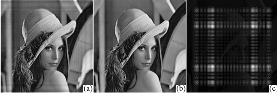
Figure 3.5: Amplitude reconstruction using the regularization by truncation, Eq. (3.55), for noiseless data \sigma=0 and z = 1.15 \cdot z_f . The reconstruction is performed for different number of singular values \tau_x = \tau_y : (a) \tau_x=210 , RMSE=0.0294; (b) \tau_x=233 , RMSE=0.0118 (c) \tau_x=235 , the reconstruction fails.
