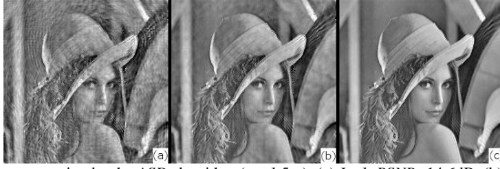
FIGURE 4. The phase reconstruction by the ASD algorithm ( z_j=1.5 \cdot z_f ): (a) L=1 , PSNR=14.6 dB; (b) L=2 , PSNR=15.5 dB; (c) L=10 , PSNR=16.3 dB.
