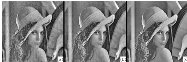
FIGURE 3. The phase reconstruction by the MF-DDT algorithm ( z_1 = 1.5 \cdot z_f ): (a) L = 1 , PSNR = 15.9 \text{ dB} ; (b) L = 2 , PSNR = 16.3 \text{ dB} ; (c) L = 10 , PSNR = 16.8 \text{ dB} .
